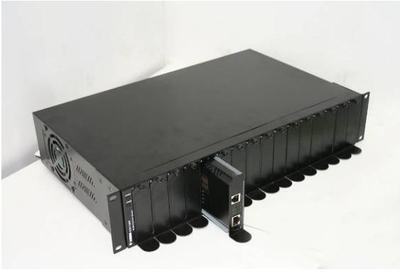
Carefully slide in the carrier until it is fully and firmly fit the chassis. Fasten the screws onto the carrier.
