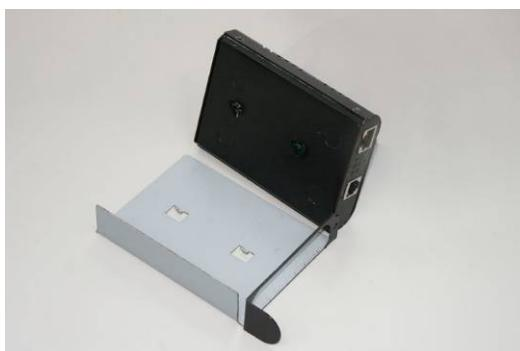
Step 2- Fit LB300A-R2, Ethernet Extender onto the carrier.
