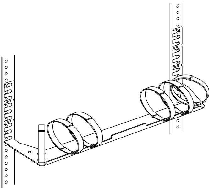
**Figure 2-1. Typical Installation of the Cable Manager.**
