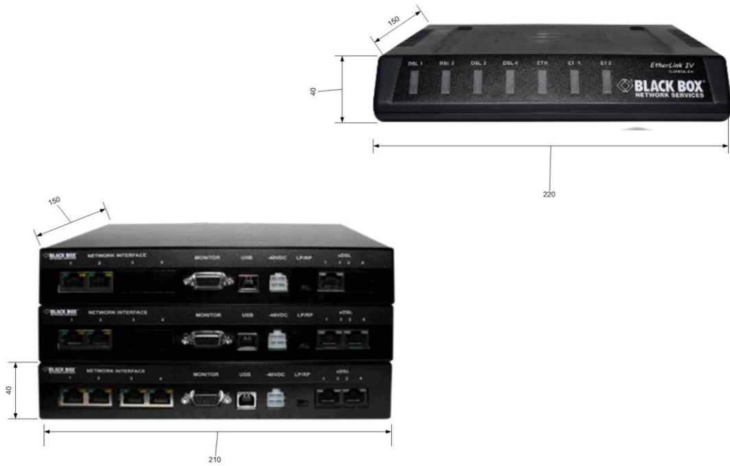
Figure 3.9 Dimension of the ABS and DIN-Rail metal enclosures.
