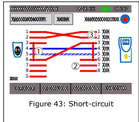
Figure 43: Short-circuit
