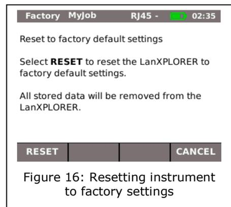
Figure 16: Resetting instrument to factory settings
