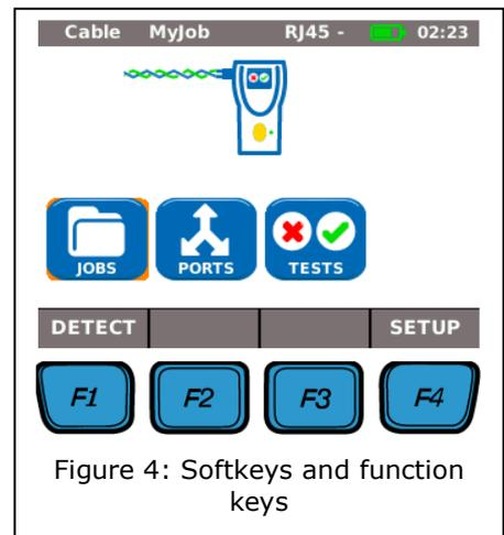
Figure 4: Softkeys and function keys
