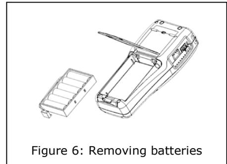
Figure 6: Removing batteries
